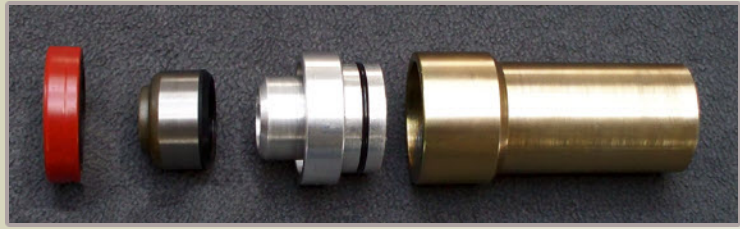
The 4T40E uses one of the most challenging axle seal designs.
